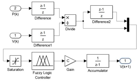
Figure 8. The implementation of the Fuzzy Logic Controller based MPPT
