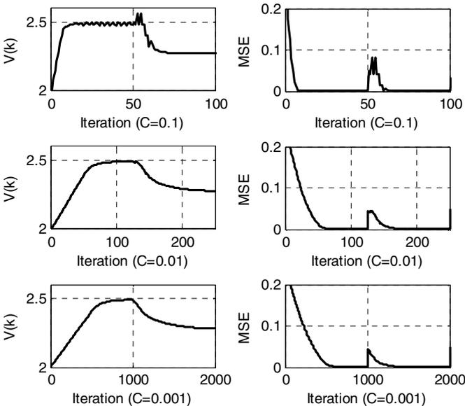
Figure 11. Control voltage and MSE error for Fuzzy Logic based MPPT
