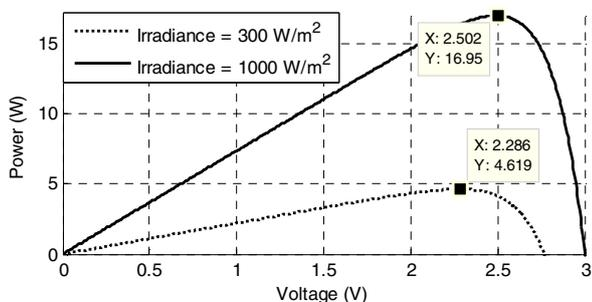
Figure 1. Power vs. voltage characteristic of a solar panel
