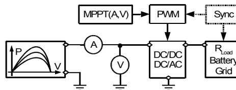
Figure 2. A common solar energy harvesting setup
