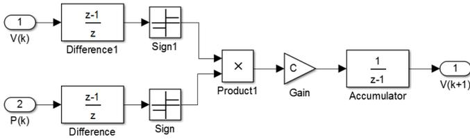
Figure 7. The implementation of the Perturb and Observe algorithm
