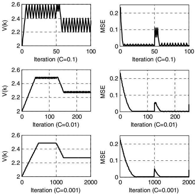
Figure 10. Control voltage and MSE error for Perturb and Observe MPPT
